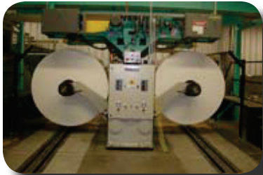
Shown here is a Roll-Rite Rollstand positioned under a boxboard converting line. Far right photo shows Roll-Rite Rollstand under a FUMA automated splicer.
