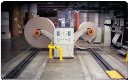
The E-Z Load Track and Trolley systems with lateral side-shifting are standard with every Roll-Rite™ Rollstand.
